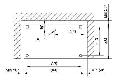
A: Minimum 850mm electrical cable over the floor.
