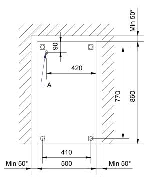
A: Minimum 850mm electrical cable over the floor.
