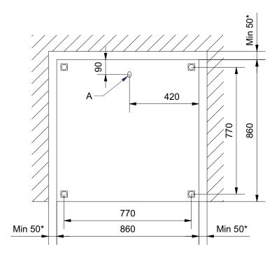
A: Minimum 850mm electrical cable over the floor.
