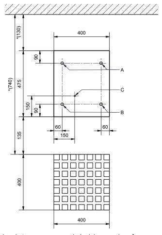
Measurements given in brackets are recommended minimum values for reasons of service and cleaning. Dimensions indicated with "\*" it is recommended to add 100 mm.
